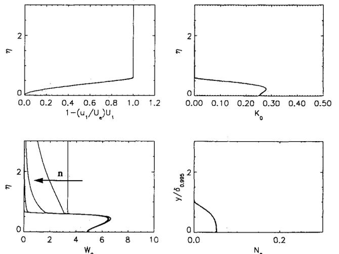
Fig. 3 Solutions of the far wake equations with different freestream values for  $W_0$ ,  $W_f = W_a 10^{-n}$ ,  $n = 0, 1, 2, 3, \dots$ ,  $2\sigma N_0(1/K_0) (dK_0/d\eta) (dW_0/d\eta)$  is included in the  $W_0$  equation.
