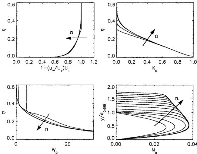
Fig. 1 Solutions of the defect layer equations with different freestream values for  $W_0$ ,  $W_f = W_a 10^{-n}$ ,  $n = 0, 1, 2, 3, \dots$
