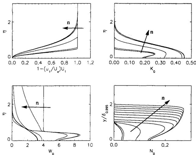
Fig. 2 Solutions of the far wake equations with different freestream values for  $W_0$ ,  $W_f = W_a 10^{-n}$ ,  $n = 0, 1, 2, 3, \dots$
